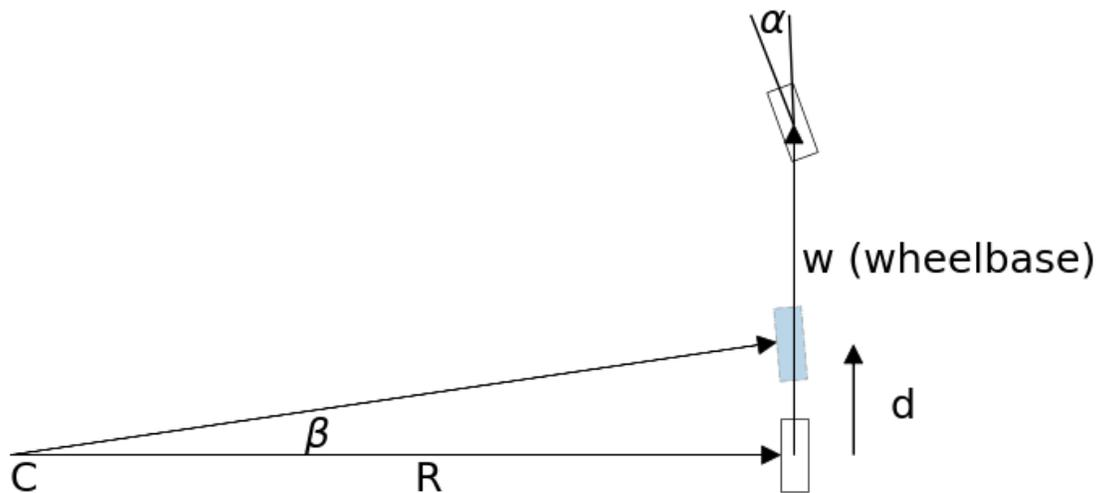
Here we see the front tire is pointing in direction  $\alpha$  relative to the wheelbase. Over a short time period the car moves forward and the rear wheel ends up further ahead and slightly turned inward, as depicted with the blue shaded tire. Over such a short time frame we can approximate this as a turn around a radius  $R$ . We can compute the turn angle  $\beta$  with
