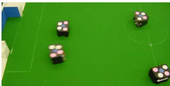
Fig. 8. A robot (lower left) navigating at high speed through a field of static obstacles.
