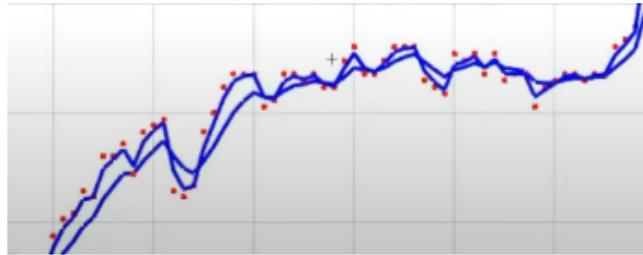
Figure 7: 1° order low pass filter,  $\alpha = 0,3$
