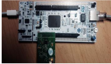
Fig. 9. Demo Base Station using STM32F767 Nucleo-144 Development Board
